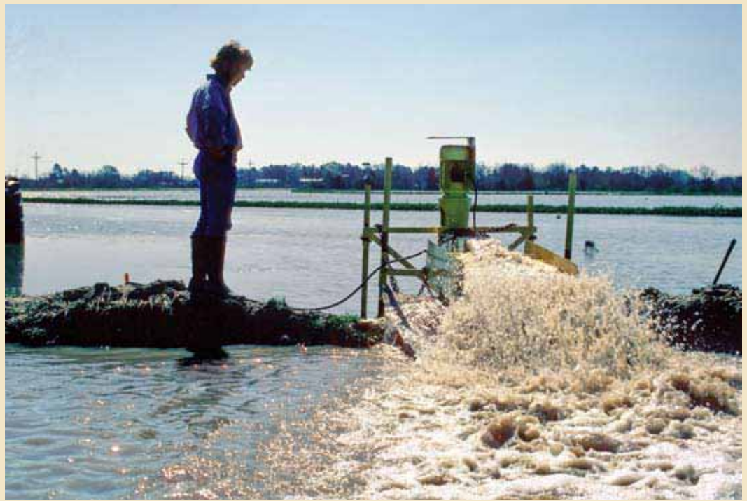
Figure 4.3. Many crawfish ponds can be adapted to allow for circulation using one or more re-lift pumps.
