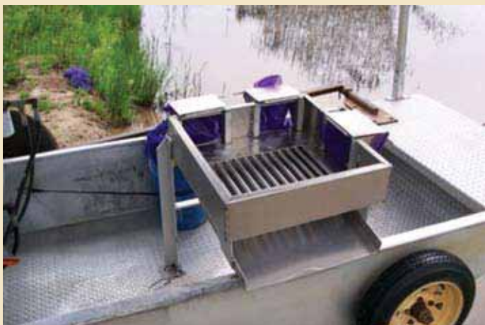
Figure 8.8. Typical shop-built "in-boat" grader designed to allow submarketable crawfish to be returned to the pond immediately after harvest via a chute placed below the parallel bars.
