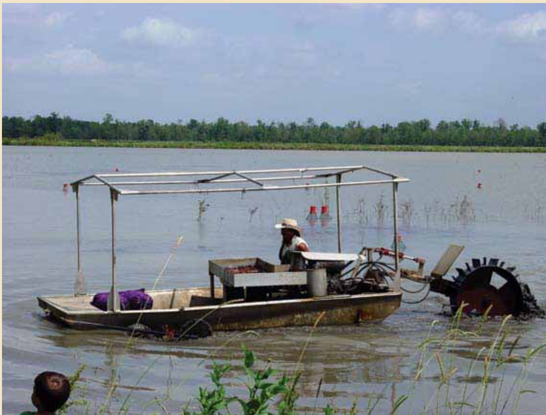
Figure 8.7. Crawfish harvesting boat powered by rear-mounted hydraulic wheel.
